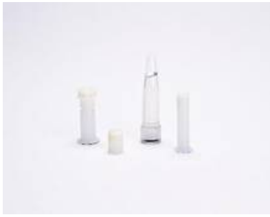
Figure 2: Unyvero sample tube, sample tube cap, sample pre-treatment tool and Master Mix tube
