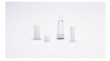
Figure 2: Unyvero sample tube, sample tube cap, sample pre-treatment tool and Master Mix tube
