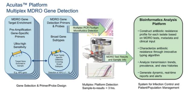
Acuitas MDRO test products combine Fluidigm microfluidic-based production genomics technology with DNA probe reagents designed and manufactured to power our CLIA lab-based Acuitas gene tests.
